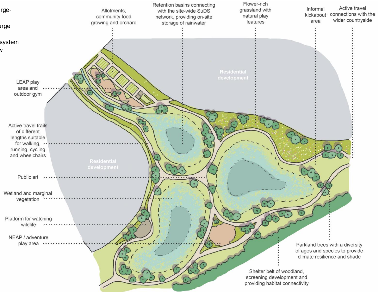
Figure 10: How large-scale retention basins can be incorporated into the design of residential schemes.
